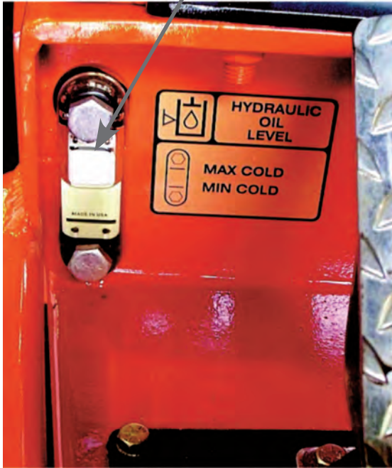
Hydraulic oil level
